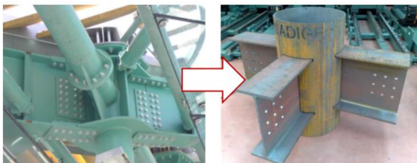
Figure 2.23: LASTEICON I-beam-to-CHS-column joint specimen (FELDMAN 2016).
