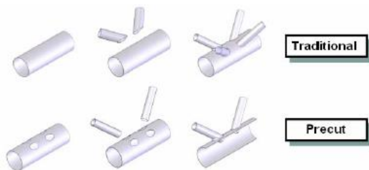
Figure 2.17: Traditional and pre-cut method for CHS joints (P. BOERAEVE, et al. 2006).
